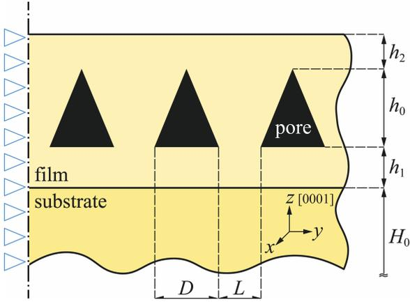
**Fig. 1.** Schematic representation of the cross section of AlN/Al<sub>2</sub>O<sub>3</sub> heterostructure with porous film.  $L$  is the distance between neighboring pores,  $D$  is the base of the pore,  $h_0$  is the pore height,  $h_1$  is the distance between the pore and the film surface,  $h_2$  is the distance between the pore and the film/substrate interface,  $H_0$  is substrate thickness. Symmetry boundary condition  $u_y = 0$  is shown with blue triangles.
