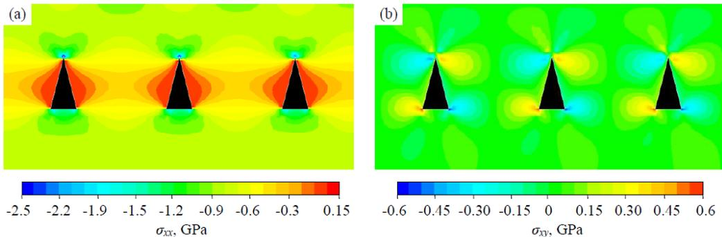
**Fig. 2.** Distributions of stress components in AlN porous film. Frame (a) shows normal stress tensor component  $\sigma_{xx}$ , frame (b) shows shear stress tensor component  $\sigma_{xy}$ .
