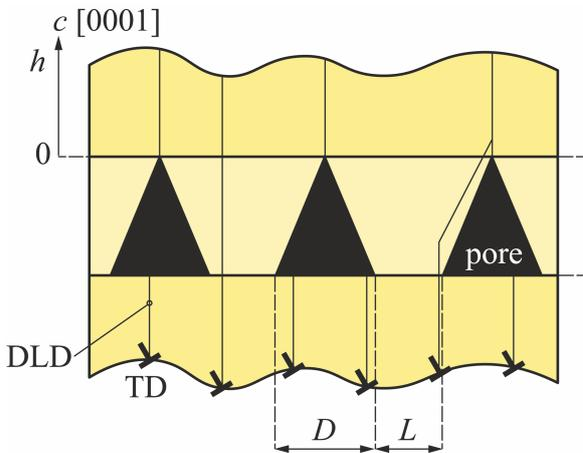
**Fig. 3.** Schematic representation of the cross section of a porous AlN film with TDs.  $h$  is the current film thickness above the porous layer. DLD is dislocation line direction threading dislocation (TD).
