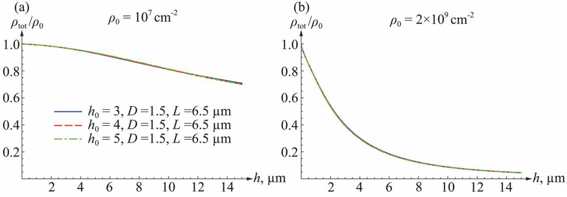
**Fig. 4.** Dependences of the normalized TD density  $\rho_{\text{tot}}/\rho_0$  on the AlN film thickness  $h$  above the porous layer. (a) initial density of TDs  $\rho_0 = 10^7 \text{ cm}^{-2}$  and (b)  $\rho_0 = 2 \times 10^9 \text{ cm}^{-2}$ . The solid, dash and dash-dotted curves correspond to the dependence obtained at a pore height  $h_0 = 3, 4$  and  $5 \mu\text{m}$ , respectively. Pore base  $D = 1.5 \mu\text{m}$ , distance between neighboring pores  $L = 6.5 \mu\text{m}$ .
